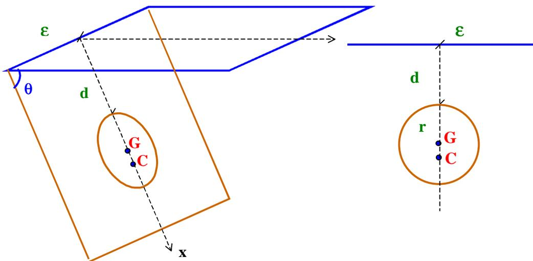
$$p = p_G \cdot \omega = \gamma \cdot z_G \cdot \omega = \gamma \cdot \text{sen } \theta \cdot x_G \cdot \omega$$
